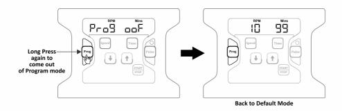
**NOTE:** On every restart, the device automatically comes out of program mode. It shows the last run default speed and time value.
