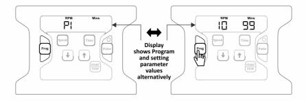
Press the "Program" button to select any program from "P1 to P9". Programs can also be selected by pressing "increment or decrement" button. Once the desired program is selected, press the "speed button" to select and set speed value. Press "Time" to select and set time value.
